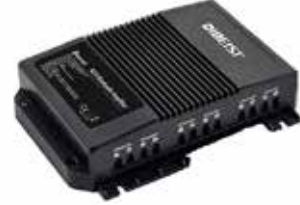
SR14145 SoundPower Bluetooth'lu Amfi BT105 6 Kanallı ( 4x30W + 2x60W ) • 12V
